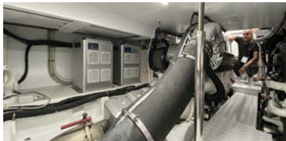
ANG ISO-BOOST™ 2x25kVA Installation on Sanlorenzo Yachts SX88
